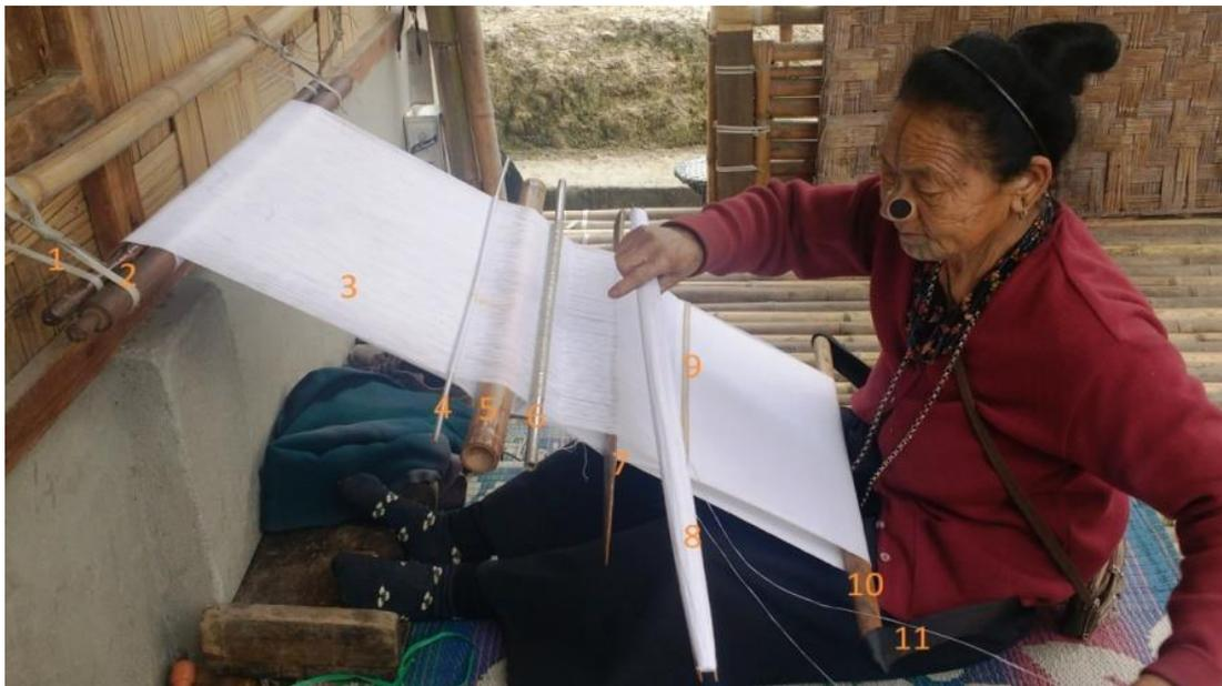
**Plate 12: Different parts of traditional loom**
