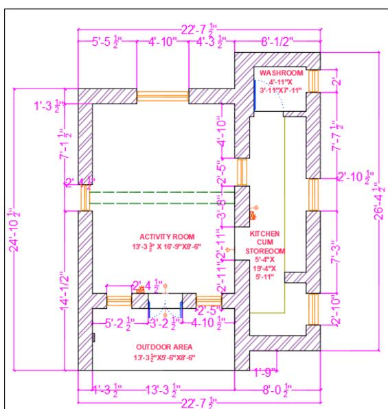
Fig.-4 Existing Floor Plan of Design
