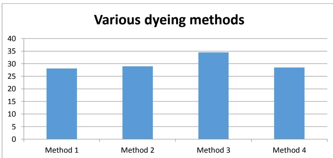
**Figure 2: Effect of Different methods of Dyeing on Colour Strength (K/S) on Jute using Sappan wood**
