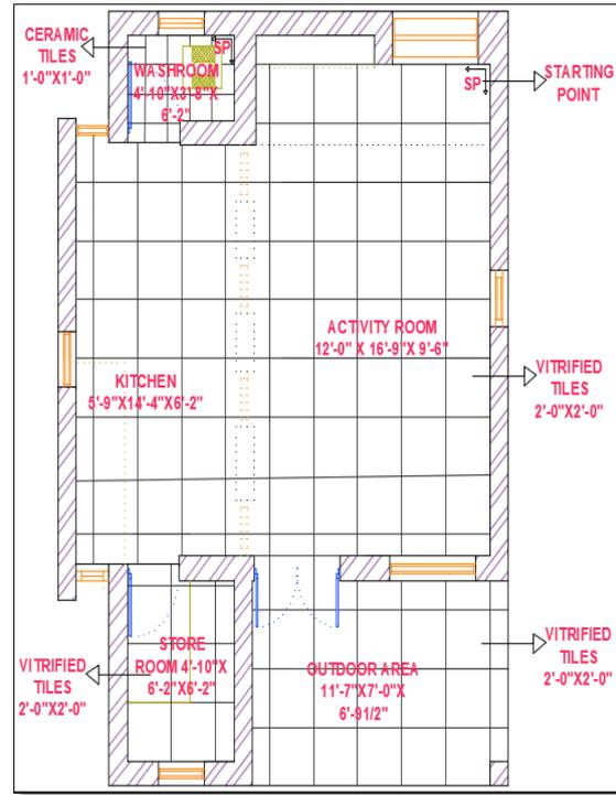
Fig.-9 Proposed Floor Plan & Flooring Layout of Design Project-II Nandghar Kashipura
