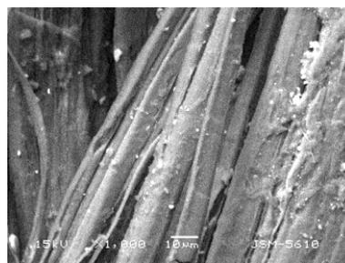
(b) Sample pretreated with copper nano colloid
