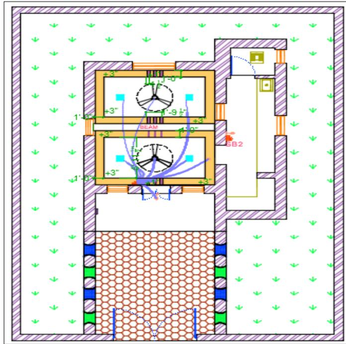
Fig.-6 Proposed False Ceiling Design and Electrical Layout of Design Project-I
