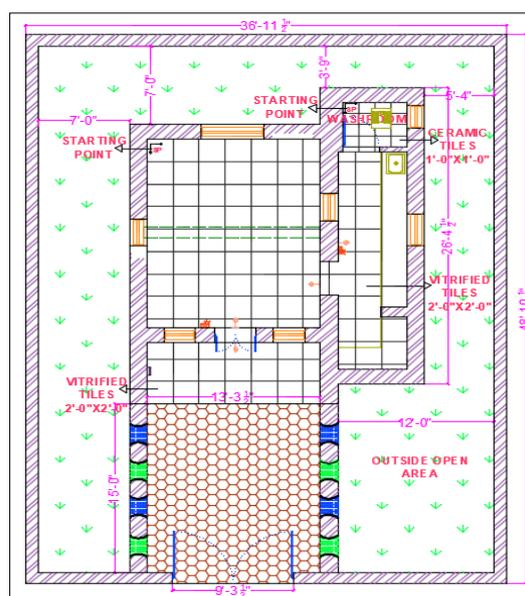
Fig.-5 Proposed Floor Plan & Flooring Layout of Design Project-I Nandghar Ujeti
