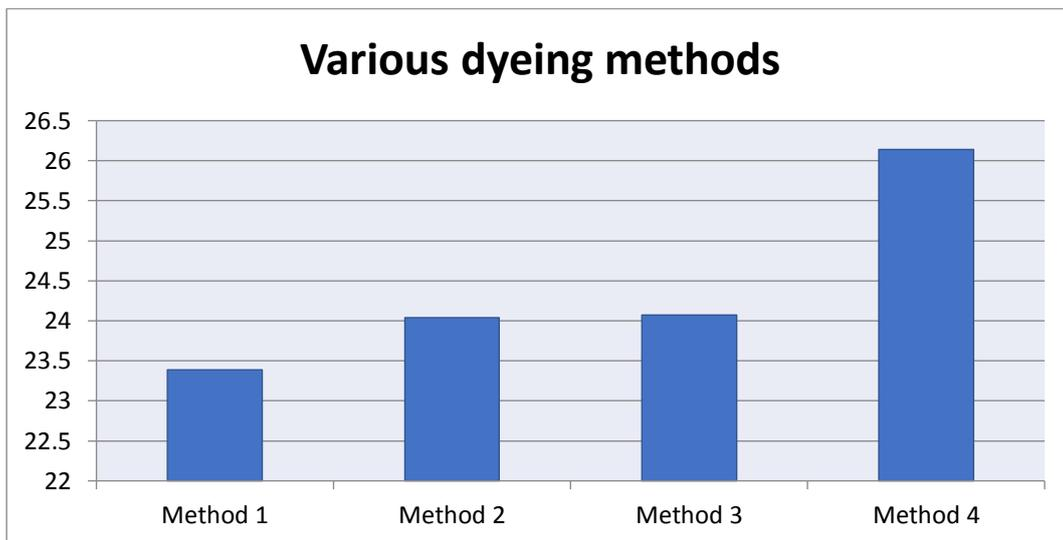
**Figure 1: Effect of Different methods of Dyeing on Colour Strength (K/S) on Jute using Turmeric**
